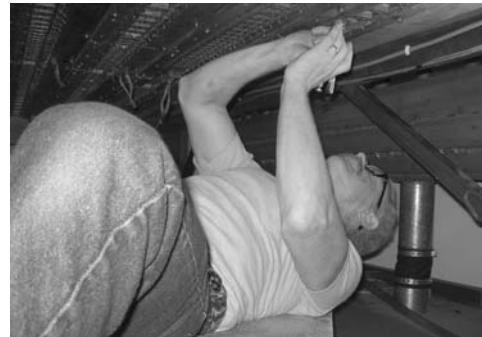
Wyatt replacing magnet cap gasket, armature and cap. The old Hope-Jones caps are prone to cipher so were replaced with newer Wurlitzer adjustables.
