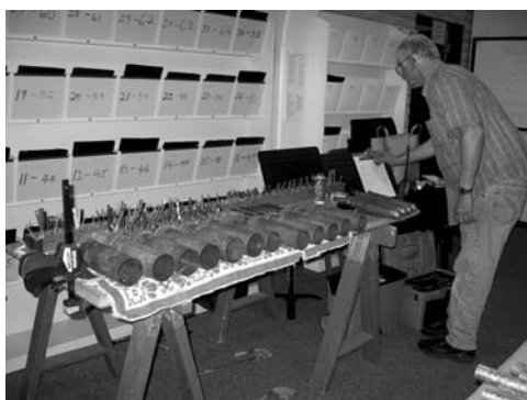
Note the size of the 25" wind pressure Tuba Mirabilis boots and shallots! Clint cleaned and polished all of the reeds and shallots. This Tuba has fire!
